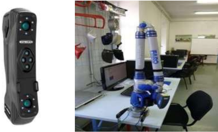
FIG.3. Simscan and FARO Platinum Arm with Laserscan Arm [16], [18]
